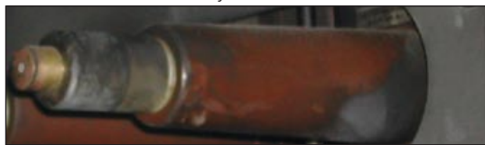
Resulting damage caused by an inexperienced PD survey.
