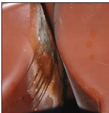
View of multiple PD sites - note the visual signs of nitric acid, a by-product of PD
