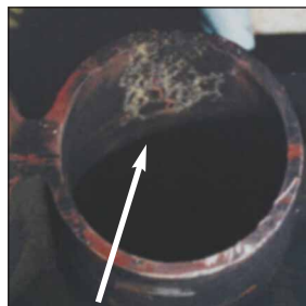
This localised Partial Discharge.....will lead to this
