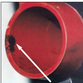
This localised Partial Discharge.....will lead to this
